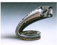
For flush free pump service with virtually leak free performance, contact the factory for specific recommendations. Carbon jacketed graphite packing used as an anti-extrusion or bull ring in high pressure pumps and valves as well as an anti-abrasion bottom ring in slurry applications. Commonly used in steam & chemical applications.
