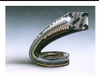
For flush free pump service with virtually leak free performance, contact the factory for specific recommendations. Carbon jacketed graphite & Kevlar packing used as an anti-extrusion or bull ring in high pressure applications, also as an anti-abrasion bottom ring in slurry applications. Commonly used in steam & chemical applications.
